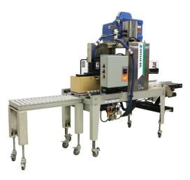
The BEL450 is a semi-automatic poly bag inserter/case former & pack station with top & bottom case taping that runs at speeds of up to 15 cases per minute. Designed for bulk filling lines, the BEL450 bag inserter/case former provides a cost effective alternative to the difficult process of manually inserting poly bag liners into corrugated cases.
